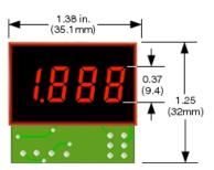
METER DEPTH: 0.95in. (24mm)
