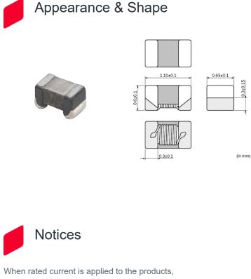
when rated current is applied to the products, inductance will be within ±30% of nominal inductance value. When rated current is applied to the products, the temperature rise caused by selfgenerated heat shall be limited to 40°C max.
