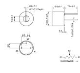
unit : mm Tolerance : ±0.3 Note: This datasheet may be out of date. Please download the latest datasheet of PV12P501A01B00 from the official website of Murata Manufacturing Co., Ltd.
