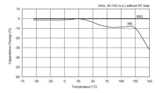
Capacitance - temperature characteristics
