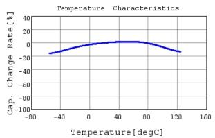
GRT033C71C104KE01 C-Temp. capchange, DC0.0V,
