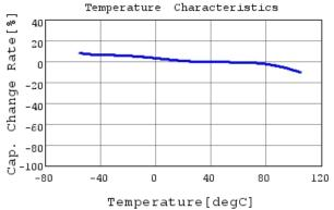
GRT155C81A105KE01 C-Temp. capchange, DC0.0V,
