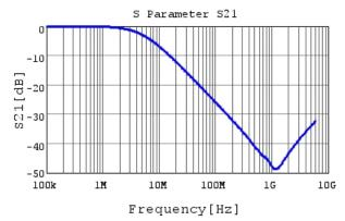
NFM15CC222D1A3 S21 DCOV,25degC, Feedthrough
