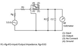
C2=10pF (including stray capacitance and input capacitance of RF Voltmeter) E1: S.S.G. Output Voltage
