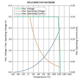
Max. Voltage, Max. Operating Voltage/Current **Reduction Curve**
