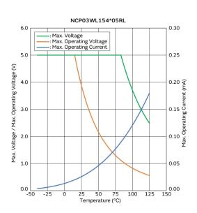
Max. Voltage, Max. Operating Voltage/Current Reduction Curve
