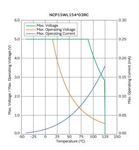
Max. Voltage, Max. Operating Voltage/Current Reduction Curve
