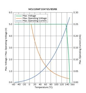
Max. Voltage, Max. Operating Voltage/Current Reduction Curve
