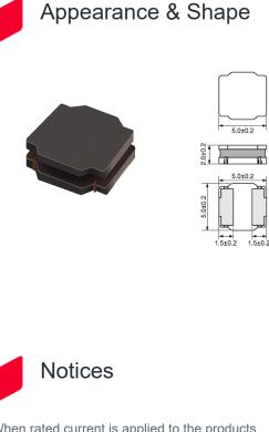
When rated current is applied to the products, inductance will be within ±30% of nominal inductance value. When rated current is applied to the products, the temperature rise caused by selfgenerated heat shall be limited to 40°C max. Keep the temperature (ambient temperature plus selfgeneration of heat) under 125°C.
