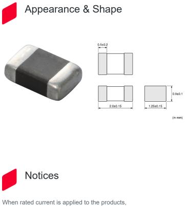
When rated current is applied to the products, inductance will be within ±30% of initial inductance value range. When rated current is applied to the products, the temperature rise caused by selfgenerated heat shall be limited to 40°C max. Keep the temperature (ambient temperature plus selfgeneration of heat) under 125°C.
