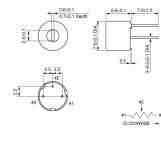
unit : mm Tolerance : ±0.3 Note: This datasheet may be out of date. Please download the latest datasheet of PV12P105A01B00 from the official website of Murata Manufacturing Co., Ltd.
