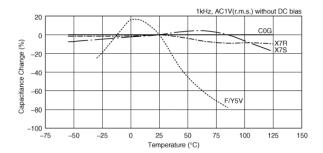
Capacitance - temperature characteristics
