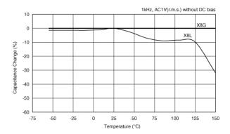
Capacitance - temperature characteristics
