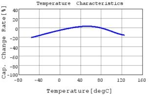
GRM21BC71C106KE11 C-Temp. capchange, DC0.0V,
