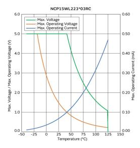
Max. Voltage, Max. Operating Voltage/Current **Reduction Curve**
