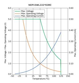
Max. Voltage, Max. Operating Voltage/Current **Reduction Curve**
