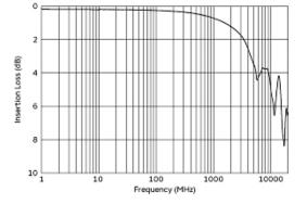
Common Mode Insertion Loss Characteristic (Typical Value)
