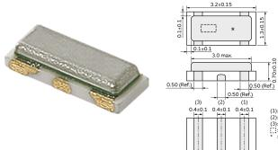
0.4±0.1 (1): Input (2): GND (3): Output Frequency Marking EIAJ Monthly Code 0.4±0.1\_ (in mm) 1.2±0.1 1.2±0.1
