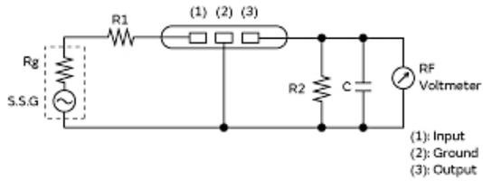
Rg-R1=R2=Input and Output Impedance
