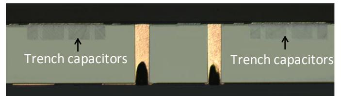
Figure 6: Cross sectional view of a silicon interposer with TSVs and High Density Capacitors (trench capacitors).
