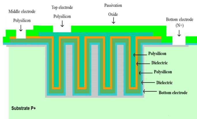
Figure 2: cross sectional view of the MIMIM architecture.
