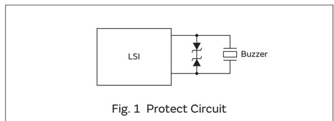
Fig. 1 Protect Circuit
