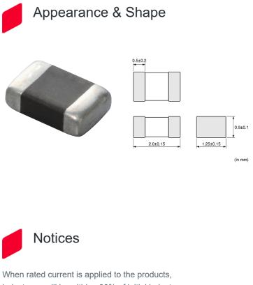
inductance will be within  $\pm 30\%$  of initial inductance value range. When rated current is applied to the products, the temperature rise caused by selfgenerated heat shall be limited to 40°C max. Keep the temperature (ambient temperature plus selfgeneration of heat) under 125°C.
