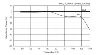
Capacitance - temperature characteristics
