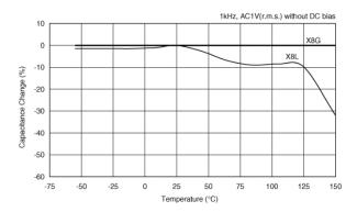
Capacitance - temperature characteristics
