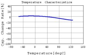
GCM155R71H104KE02 C-Temp. capchange, DC0.0V,
