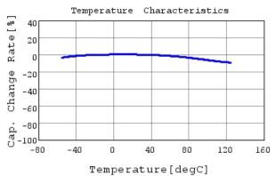
GRM21BC72A105KE01 C-Temp. capchange, DC0.0V,
