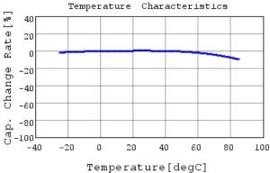
GRM31MB31A106KE18 C-Temp. capchange, DC0.0V,
