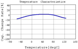
GRT155C71A105KE13 C-Temp. capchange, DC0.0V,
