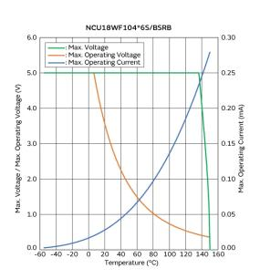
Max. Voltage, Max. Operating Voltage/Current Reduction Curve
