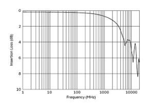
Common Mode Insertion Loss Characteristic (Typical Value)
