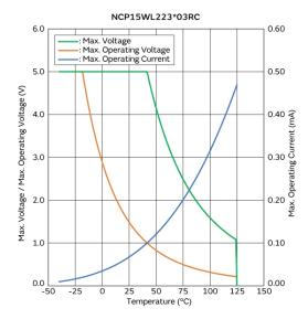
Max. Voltage, Max. Operating Voltage/Current **Reduction Curve**
