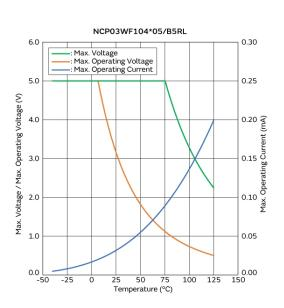
Max. Voltage, Max. Operating Voltage/Current Reduction Curve
