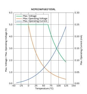
Max. Voltage, Max. Operating Voltage/Current Reduction Curve
