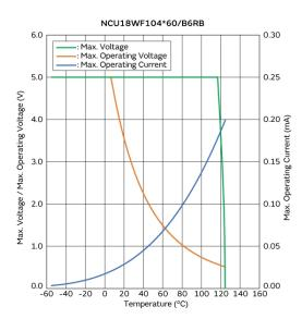
Max. Voltage, Max. Operating Voltage/Current **Reduction Curve**
