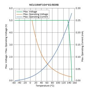
Max. Voltage, Max. Operating Voltage/Current **Reduction Curve**
