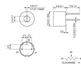
unit : mm Tolerance : ±0.3 Note: This datasheet may be out of date. Please download the latest datasheet of PV12P100A01B00 from the official website of Murata Manufacturing Co., Ltd.
