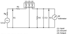
R1+Rg=R2=600 $\Omega$  ±5%, Rg=50 $\Omega$ C2=10pF (including stray capacitance and input capacitance of RF Voltmeter) E1: S.S.G. Output voltage
