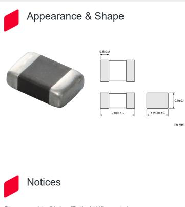
Please consider 'Notice (Rating).' When rated current is applied to the products, inductance will be within ±30% of initial inductance value range When rated current is applied to the products, the temperature rise caused by self-generated heat shall be limited to 40°C max.
