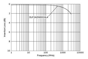
**Differential Mode Transmission Characteristics** (Typical Value)
