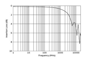
Common Mode Insertion Loss Characteristic (Typical Value)
