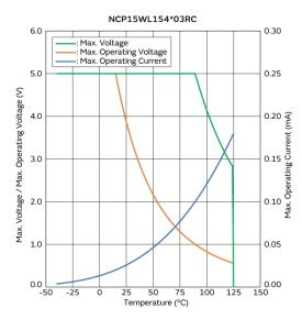
Max. Voltage, Max. Operating Voltage/Current **Reduction Curve**
