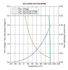
Max. Voltage, Max. Operating Voltage/Current Reduction Curve
