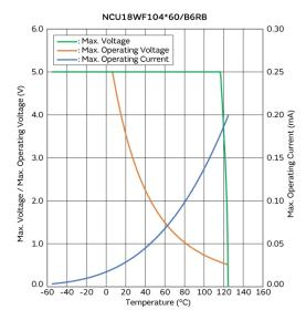
Max. Voltage, Max. Operating Voltage/Current **Reduction Curve**
