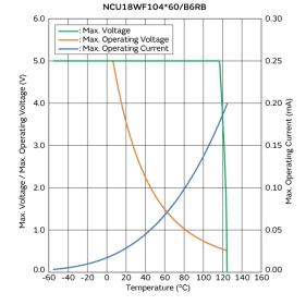
Max. Voltage, Max. Operating Voltage/Current **Reduction Curve**
