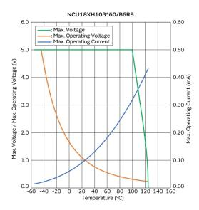
Max. Voltage, Max. Operating Voltage/Current **Reduction Curve**
