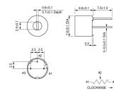
unit : mm Tolerance : ±0.3 Note: This datasheet may be out of date. Please download the latest datasheet of PV12P502A01B00 from the official website of Murata Manufacturing Co., Ltd.
